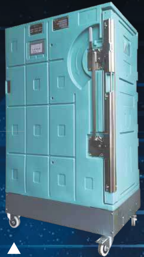
▲ 900L Olivo Roll (A420 unit) maintains 8h at -18°C with an ambient temperature at 30°C, 30h at +2°C/+8°C with an ambient temperature at 32°C and 17h at 0°C/+4°C with an ambient temperature at 43°C.
